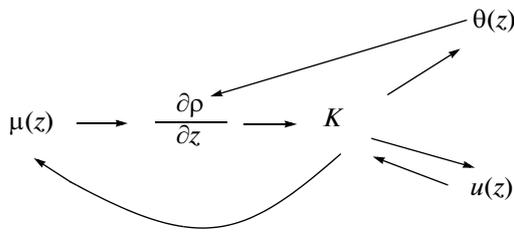
**Fig. 1.** Scheme of the main connections in the model.  $\mu(z)$  is the partial density of the heavy admixture (spray droplets),  $\rho$  is the air density, and  $K$  is the coefficient of turbulent viscosity.
