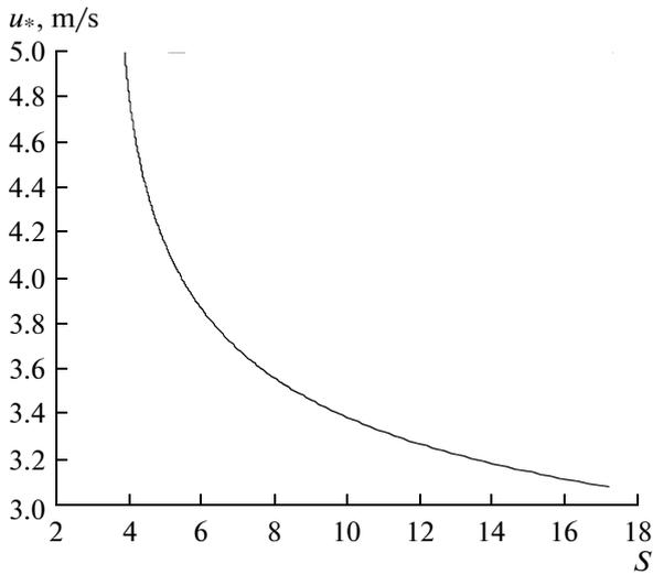
Fig. 3. Example of the dependence that the friction force has on the droplet concentration according to (25).
